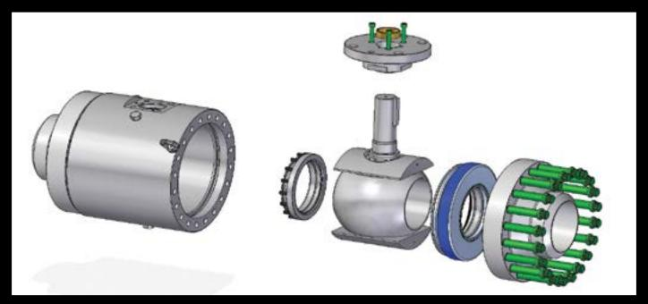
Perar Compact Ball Valves are designed according to API6A to combine a compact design with robustness and reliable performances. The valves do not rely on lubricant or grease to assist sealing between the ball and seat also when metal-to-metal sealing is used. The valve design is based on trunnion mounted or support plate configuration in order to get the operating torque as lower as possible.
