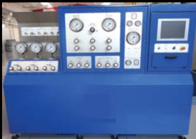
Automatic test panel for API 6A PR2 and endurance cycling tests
